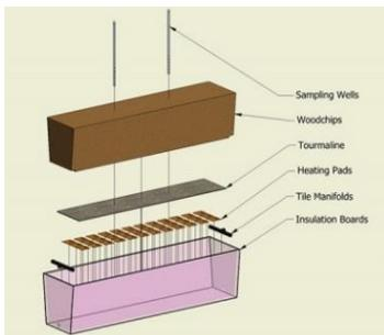
*Diagram of how the 6” x 6” heating pads fit within the woodchip bioreactor.*
