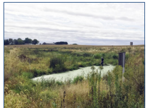
JK Thacker - Dr. Karl Rockne, University of Illinois Chicago, is taking samples in NREC's first constructed wetland for tile drainage treatment in Bureau County.
