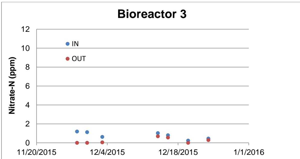
Figure 7. Nitrate concentrations in and out of Bioreactor 3 (following winter wheat/cover crops).
