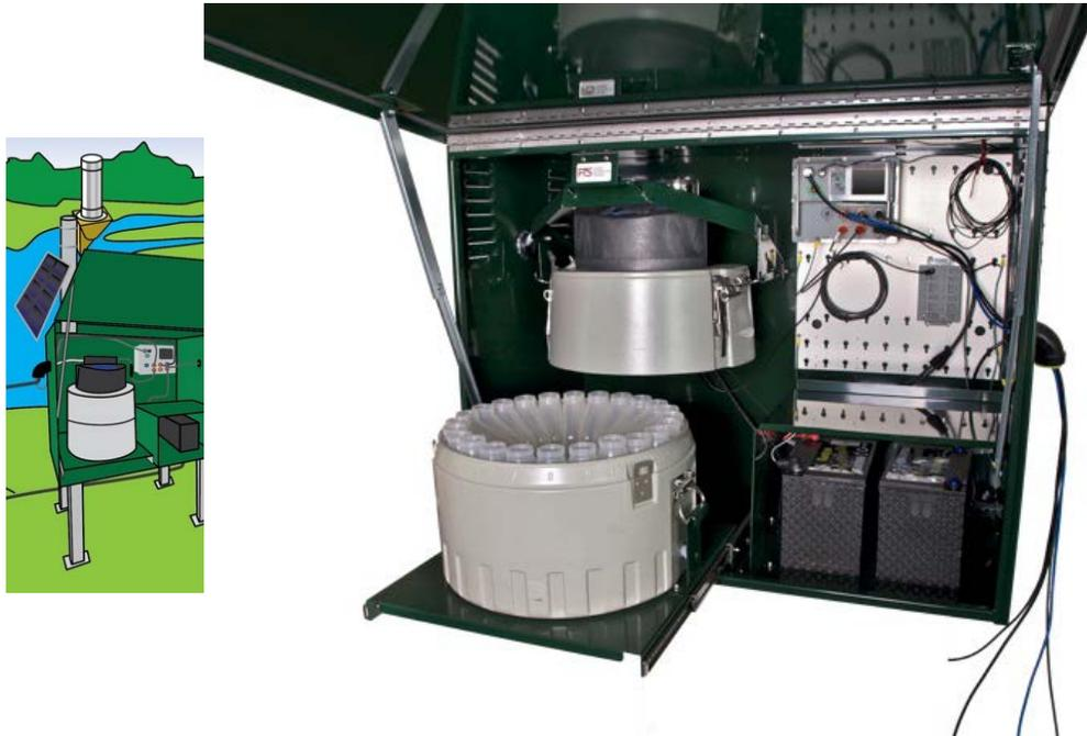
Figure 2. The enclosure with sampling equipment and datalogger, which will be placed on posts near the tile drains.
